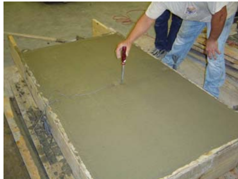
a) Embedding I-button in Slab
