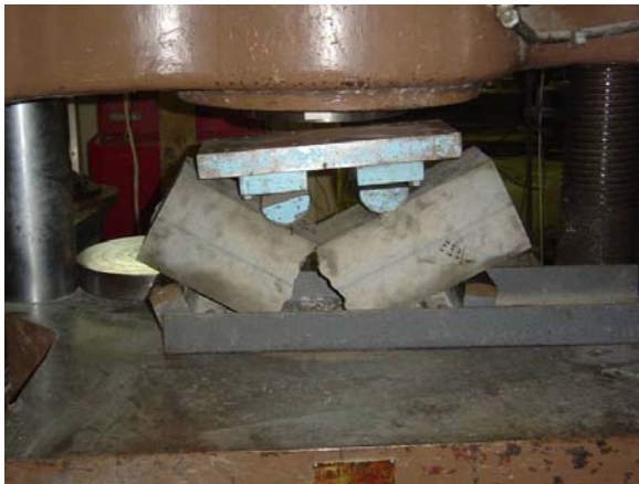
c) Flexural Strength Test
