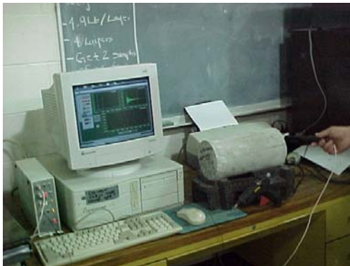
Figure 3.2 - Setup of Free-Free Resonant Column (FFRC) Test
