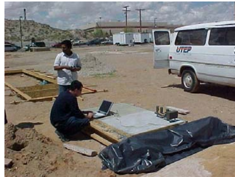
b) PSPA Test for In-place Modulus
